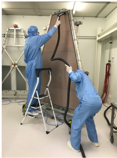
Figure 15: Vacuum cleaning of the drift panel before closing a gap.
