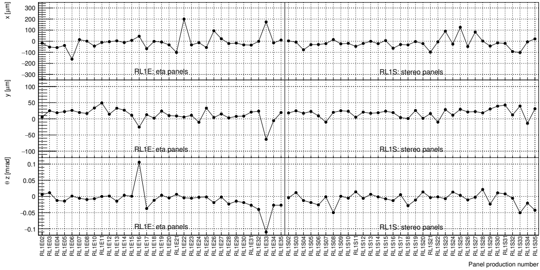
Figure 33: Metrology fit result: second layer position( x and y ) and rotation (about the z axis, \theta_z ) parameters with respect to the first layer, as a function of panel production number. The reported values are deviations with respect to the nominal layer frame, which coincides with that of its 5th PCB (see Fig. 30). The panel frame is fixed on the first layer, whose parameters are thus zero by definition, and are not reported in this plot.
