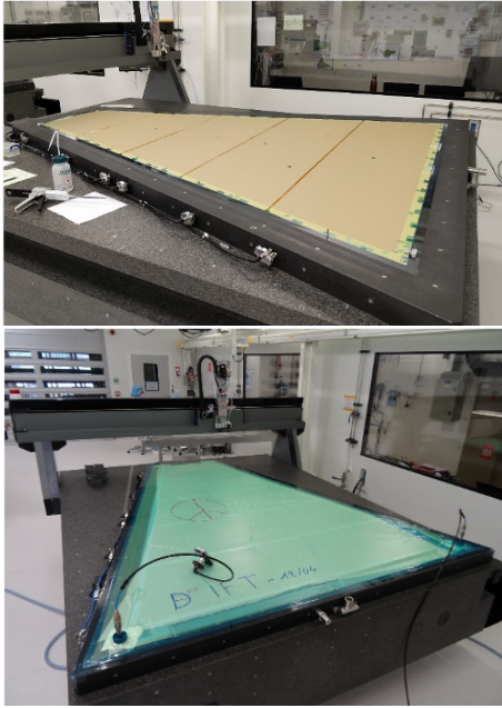
Figure 10: Panel gluing: first side (top); vacuum bag (bottom).
