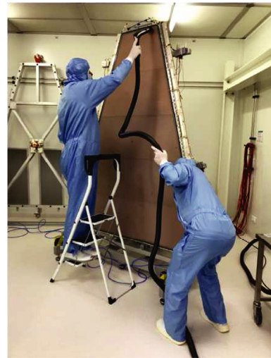
Fig. 15. Vacuum cleaning of the drift panel before closing a gap.
