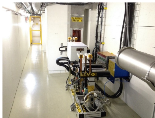
Figure 1: Irradiation tables (front) and shuttle system (back) in IRRAD.
