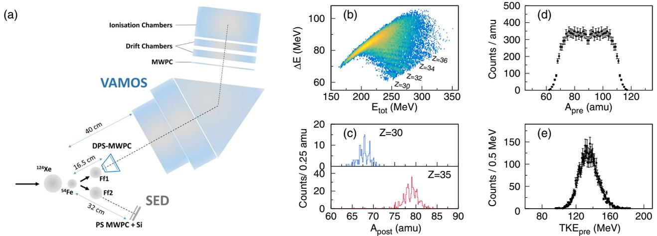
FIG. 1. (a) Schematic of the experimental setup for detecting the coincident fission partners (Ff1 and Ff2). (b) Correlation between the fragment energy loss  $\Delta E$  and total energy  $E_{\text{tot}} = \Delta E + E_{\text{res}}$  detected in VAMOS++. Some  $Z$  lines are indicated for reference. (c) Postneutron  $A$  distributions for selected  $Z$  values. Preneutron (d)  $A$  and (e) TKE distributions.
