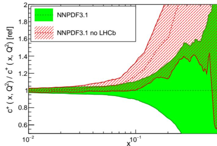
Current LHCb data provides powerful constraints on the quark PDFs at high- $x$
