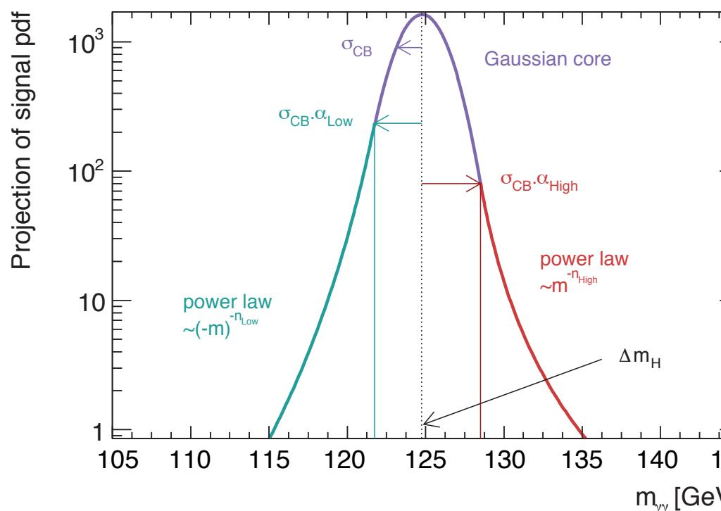
"SM Higgs" peak and signal modelled with double-sided Crystal Ball function (gaussian core and power laws in the tails)
