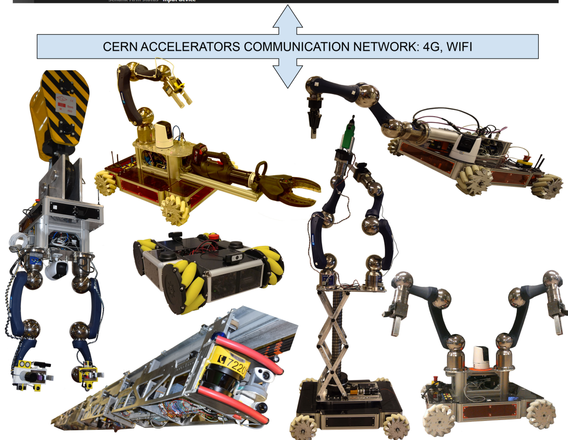
Figure 3. Set of modular robots developed at CERN-EN-SMM-MRO section to perform safe operations in radioactive and hazardous scientific facilities (i.e., Cranebot, Charmbot, CERNBot, CERNBot2, TIM, and Unified GUI).
