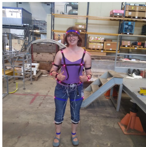
(b) One of the authors wearing the LEDs to calibrate the system and test for occlusions. Velcro strips were used to attach the LEDs to the body.
