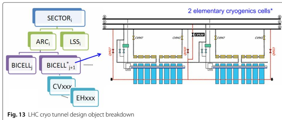
**Fig. 13** LHC cryo tunnel design object breakdown
