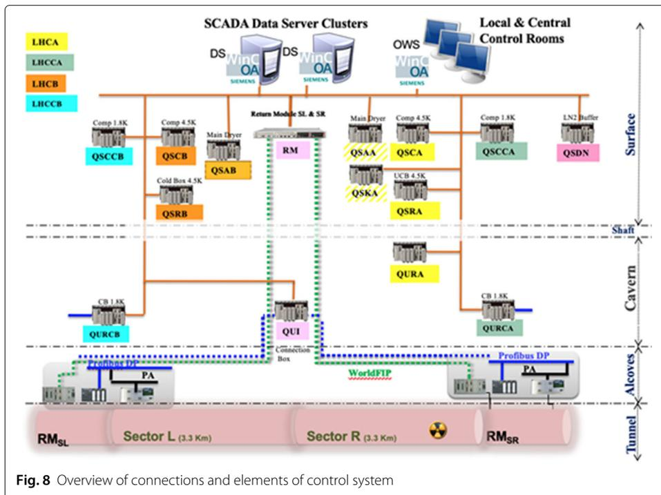
Fig. 8 Overview of connections and elements of control system
