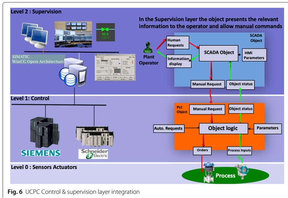
Fig. 6 UCPC Control & supervision layer integration
