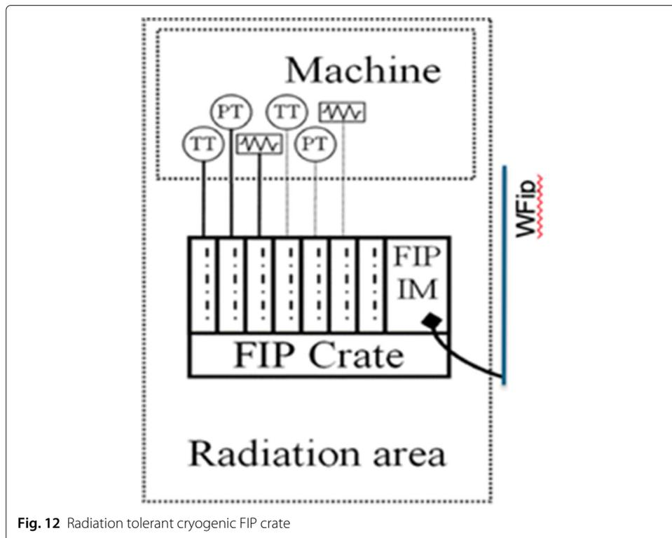
**Fig. 12** Radiation tolerant cryogenic FIP crate
