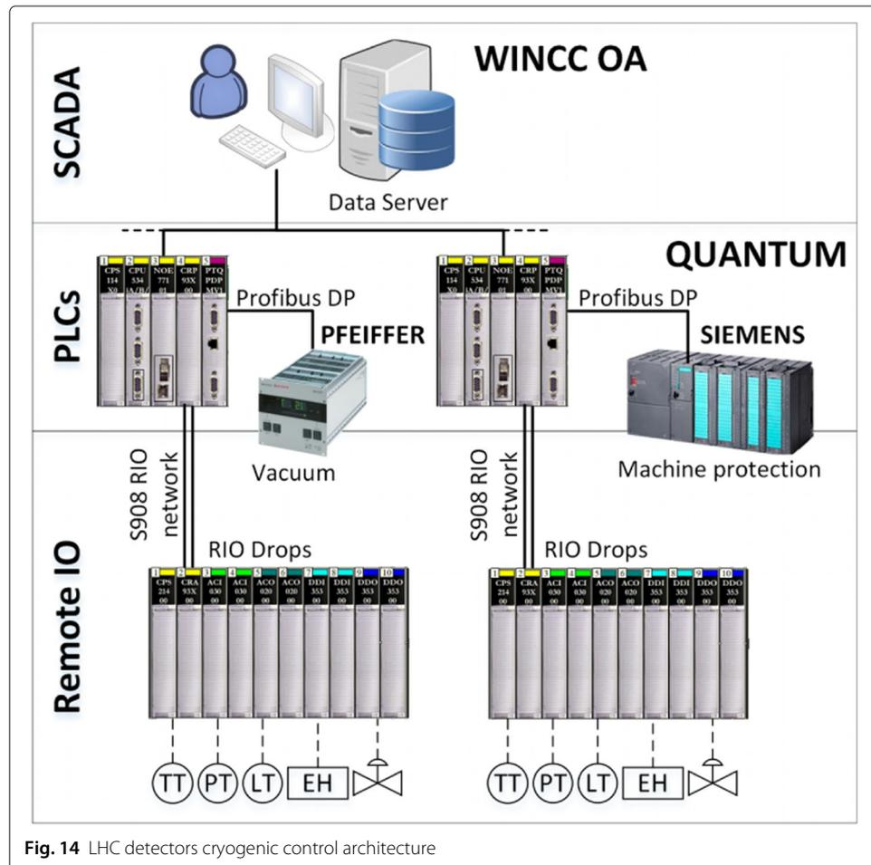
**Fig. 14** LHC detectors cryogenic control architecture
