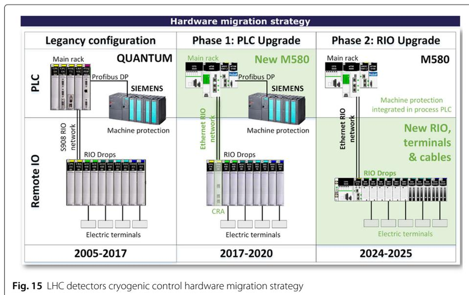
Fig. 15 LHC detectors cryogenic control hardware migration strategy
