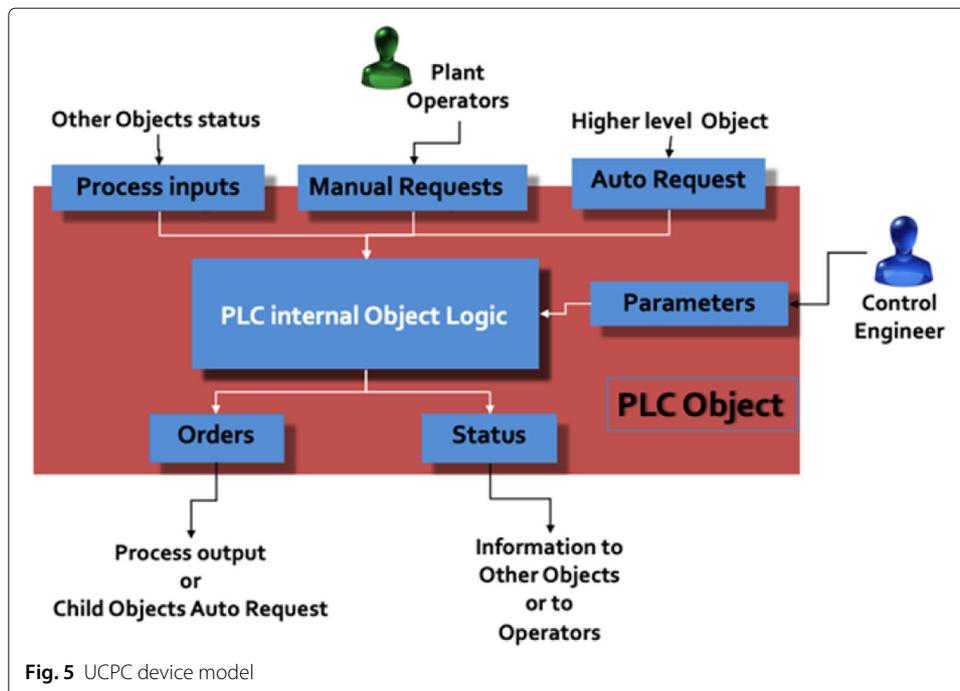
Fig. 5 UCPC device model
