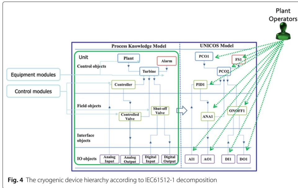
Fig. 4 The cryogenic device hierarchy according to IEC61512-1 decomposition
