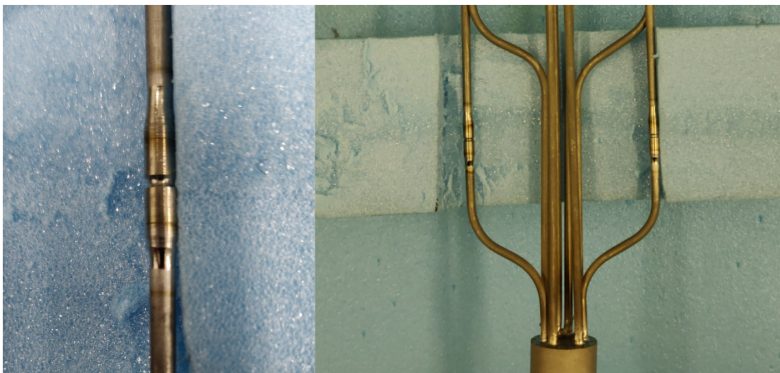
Figure 14. Photographs of welds from the demonstration ATLAS ITK cooling circuit manifold.
