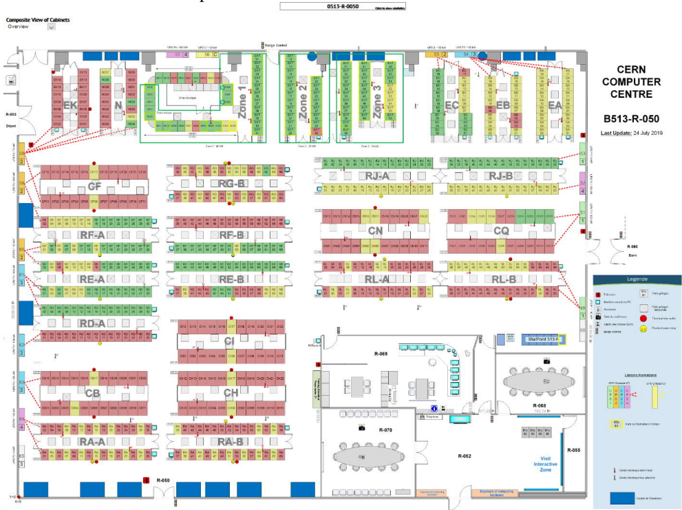
Figure 1: Schematic floor plan of R-050. The rack colours reflect the occupancy (green is empty).
