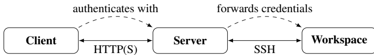
Figure 1: Schema of the three application parts and the client's authentication interactions (dashed).
