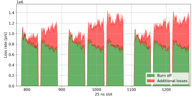
Figure 3: Bunch-by-bunch loss rate for Beam 1 at 4.2 h in SB for Fill 6666 [10].
