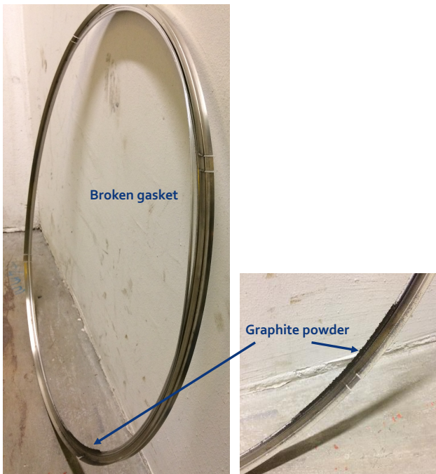
Figure 3: Example of damaged gaskets exchanged during YETS.
