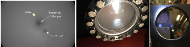
Figure 5: The damages caused by the SR to the BSRT system: the image intensifier ageing, the etching of the viewport material and the coating deterioration of the NUV band-pass filter.
