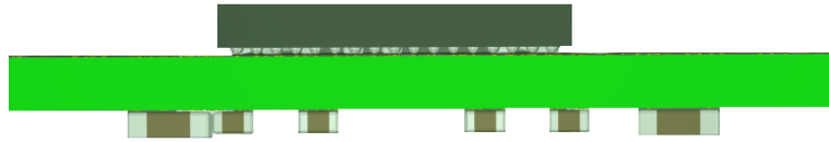
Figure 6: Side view of the chip and the decoupling capacitors position, when they are on the different layers.
