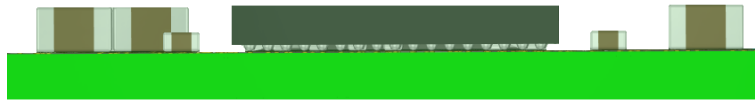
Figure 8: Side view of the chip and the decoupling capacitors position, when they are on the same layer.
