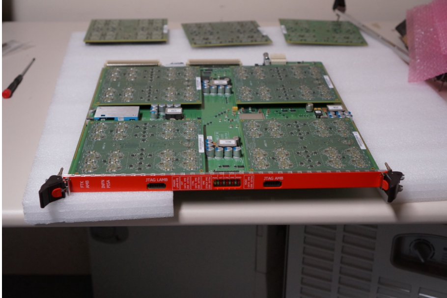
Figure 12: Photo of an Associative Memory Board with four LAMBs mounted. Additional LAMBs can be seen in the background.
