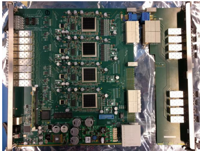
Figure 20: The FTK-to-High-Level-Trigger Interface Card (left) and its RTM (right).
