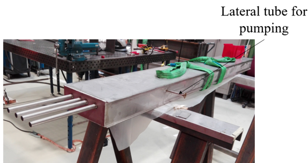
FIG. 4. The HIP capsule containing the CuCr1Zr and tubes assembly, PT and He leak tested with the lateral tube for pumping.
