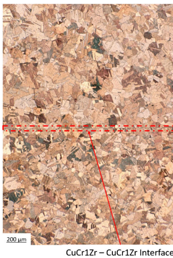
FIG. 10. Optical microscopy of a sample containing the HIP diffusion bonded CuCr1Zr-CuCr1Zr interface. The surface inspected has been mechanically polished and chemically etched.
