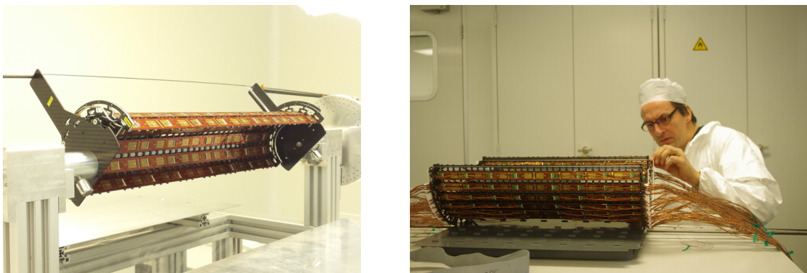
Figure 33. BPIX L2 half-shell after module mounting (left), and BPIX L4 half-shell with modules and cables (right).
