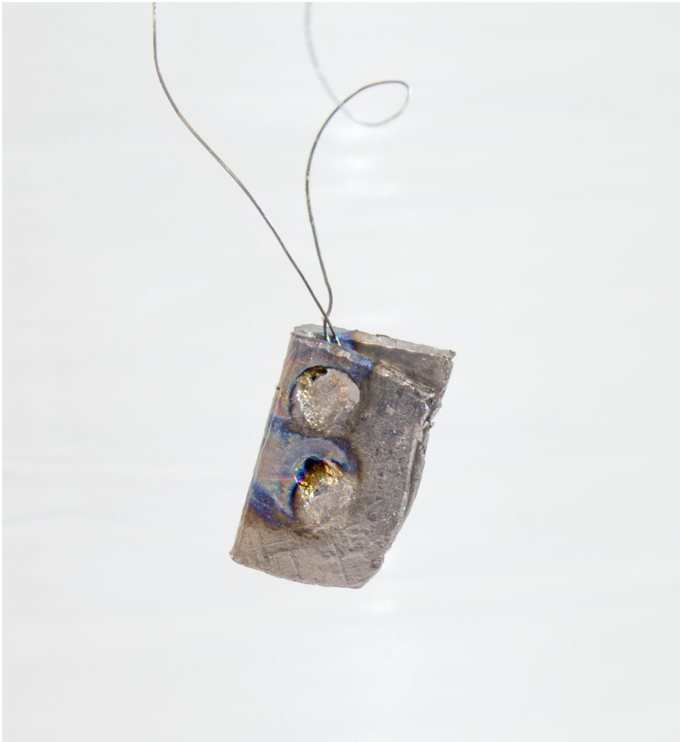
Figure 10.16: Photograph of one of the resistance welded joints. Image credit: Stefan Sellner.
