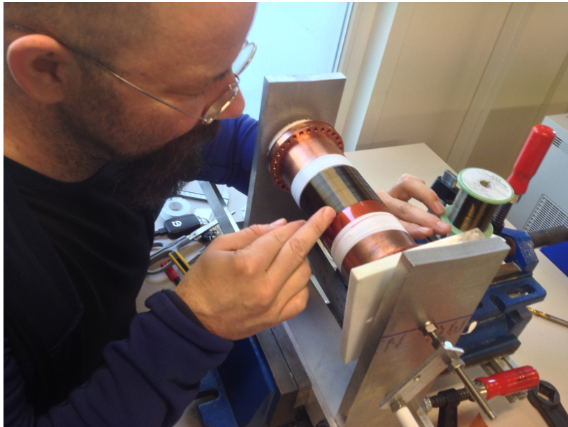
Figure 10.13: Photograph taken during the construction of the 2017 self-shielding system. The coil is being wound on a layer of Kapton sheets wrapped on the trap chamber.
