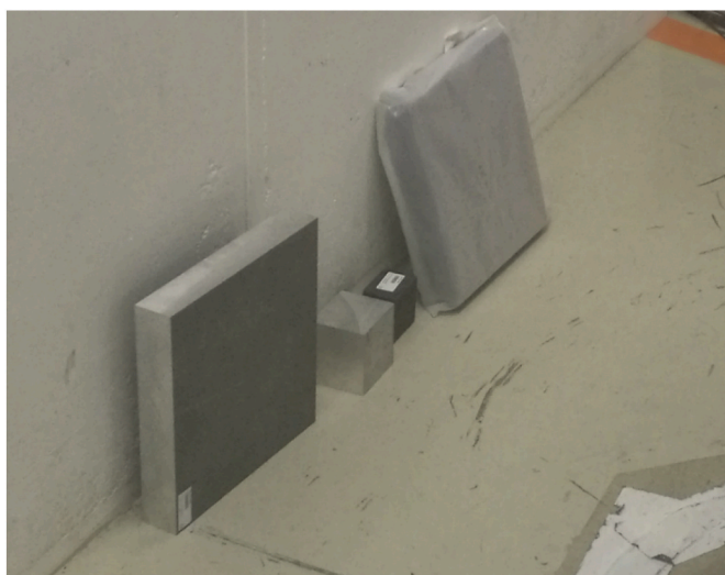
Fig. 11. Samples of Aluminum and Iron irradiated at CHARM.
