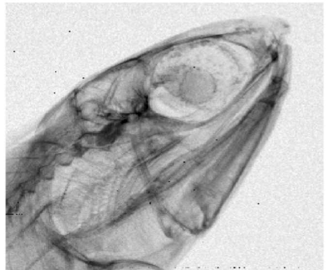
Fig. 8b. Head of the same anchovy as in Fig. 6, now using a Medipix2 assembly with a Si sensor. Much more detail is visible with the 14 \times 14 \text{ mm}^2 sensor matrix, composed of 256 \times 256 pixels (Llopert, 2007).
