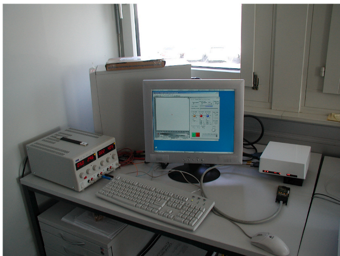
Fig. 7a. A MUROS2 readout box, right, with the small Medipix2 board in front, connected to a PC. The 100 V reverse bias voltage for the sensor is supplied externally by the power supply module, front left. [CERN, 2003 unpublished].
