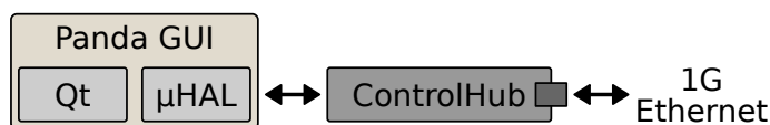
Figure 3.18: Block diagram of the Panda GUI software that is communicating with the ControlHub software using the \mu HAL library.
