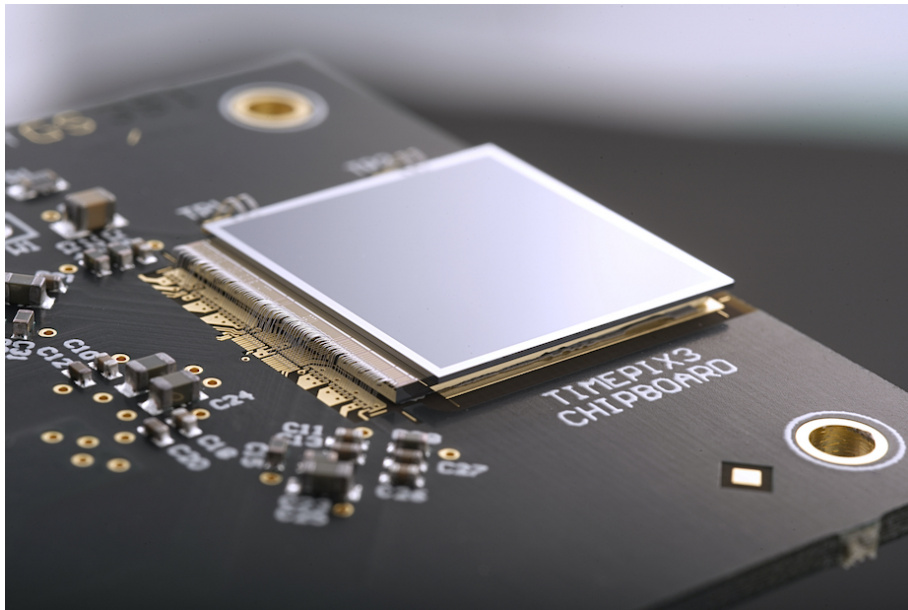
Figure 2.11: Photo of a Timepix3 hybrid pixel detector with a silicon sensor, from [47].
