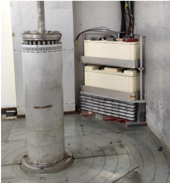
Figure 1: Photo of a ^{60}\text{Co} source in the center and the two cold boxes in the corner. Lines on the floor denote the distance from the center for which the dose rates are well-known.
