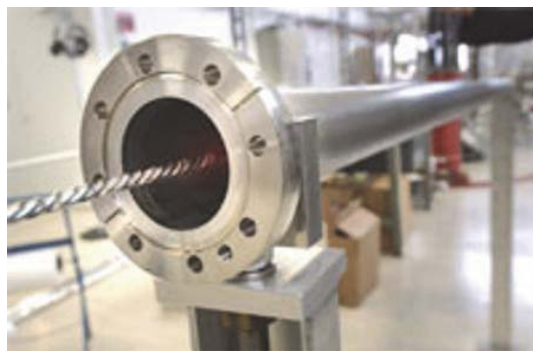
Fig. 8.14. Sputtering configuration with a cathode consisting of twisted wires.
