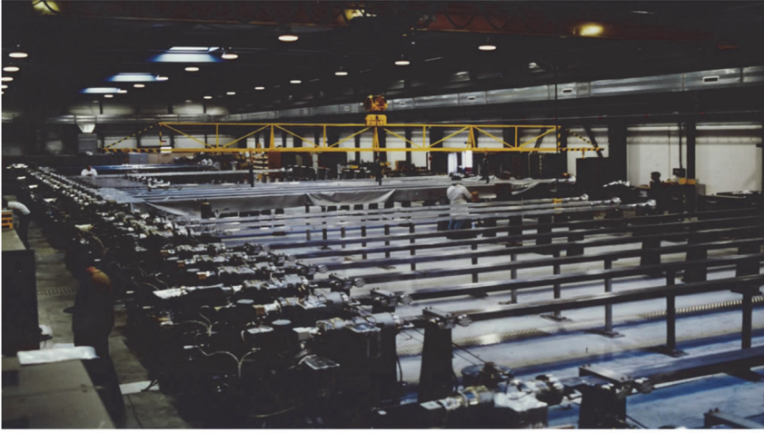
Fig. 7.11. The test laboratory of the LEP chambers. About 2000 aluminium chambers were tested in batches of 12. Only those providing a pressure lower than 2 \times 10^{-9} Pa after bake-out were accepted.
