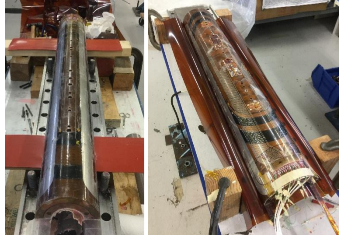
Fig. 4. Inner (left) and outer (right) potted coils with instrumentation and additional strip heaters on the coil outer surfaces.
