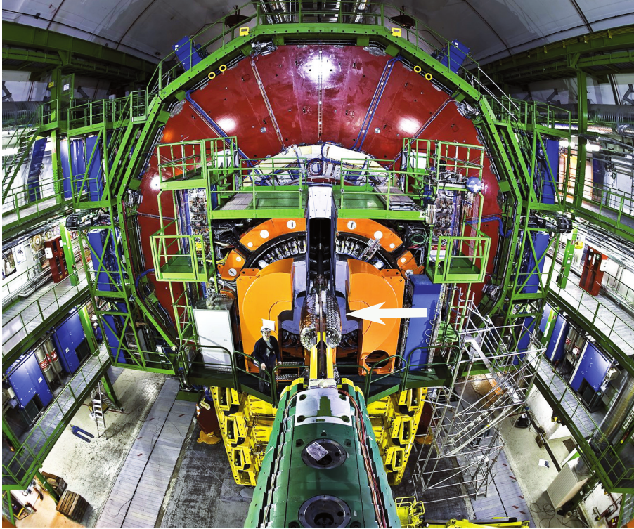
Figure 1: Picture of the forward region of the CMS experiment with the two half-cylinders of the CASTOR calorimeter (indicated by an arrow) visible in the zone where the collar shielding (orange) structures are open. The green cylindrical structure in the foreground belongs to the target absorber region. The massive shielding around the calorimeter is in the open position. The two half-cylinders of CASTOR are not yet closed around the LHC beam pipe that is visible emerging from the target absorber region in the foreground and disappearing towards the IP inside the CMS detector.
