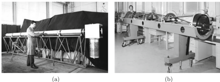
Fig. 7.15 (a) A threshold gas Cherenkov counter as used to tag particles in the secondary beams. CERN IT 6304088. (b) CEDAR counter (internal part). Here on the mounting bench. The counter is a differential Cherenkov, corrected for chromaticity, able to differentiate pions from kaons up to 350 GeV. Counters of this type were used in all SPS hadron beams. CERN PHOTO 7603033
