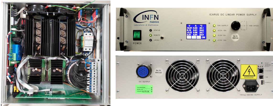
Figure 4. Inside (left) and front and rear panels (right) of the ICARUS LVPS module.
