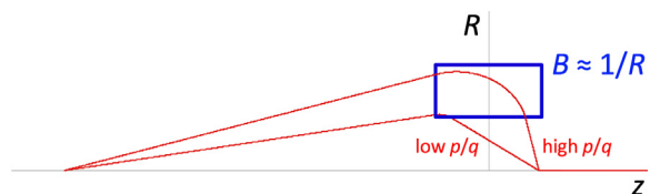
Fig. 4. A possible compensation of the effect shown in Fig. 3. Particles with different p/q , differing by the same factor 2 as in Fig. 3, and originating at the same vertex, are given different initial directions so that they travel in the thick toroidal lens over different path lengths. Ideal toroidal field with 1/R dependency. The net effect is to converge the different particles in the same point on the z -axis.
