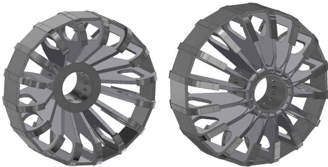
Fig. 17. Front (beam side, left) and back (patient side, right) view of the complete toroidal magnet for a proton gantry, with inner bore diameter of 0.8 m. Outer dimension is a diameter of 3.3 m, including the concept of support structure.
