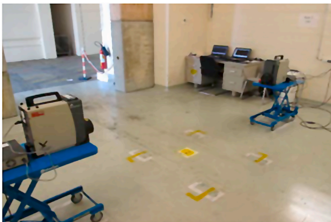
Fig. 5. Gamma spectrometry performed in a dedicated area. The white marks on the floor represent the location of the waste package.
