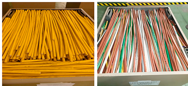
Fig. 2. Picture of a waste package from the pilot process (cables sorted by family, left) and from the current process (mixed cables, right).
