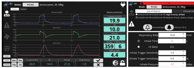
Fig. 4. Example page displays from the Native User Interface. On the left, a typical homepage, on the right, two screens showing alarms and settings. Numbers and graphs are indicative.
