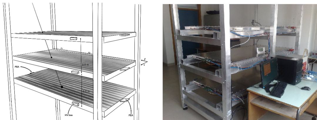
Figure 1. Left: Drawing of an EEE telescope, made of 3 MRPCs placed at 0.5 m on a support structure. Right: Picture of a typical installation in one of the school of the EEE network (ITIS Galileo Galilei in Arezzo).
