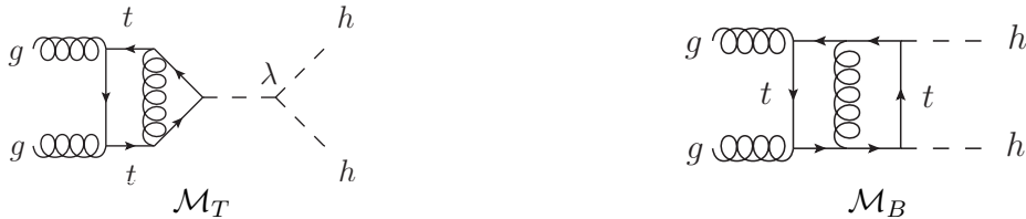
Figure 1. Triangle-like (left) and box-like (right) diagrams contribute to the full amplitude. The former contain the Higgs self-coupling, while the latter do not.
