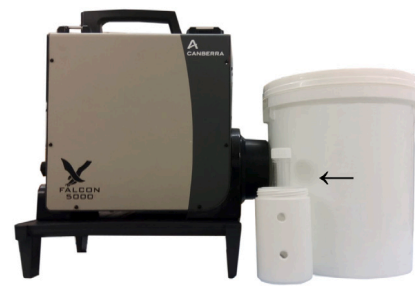
Fig. 1. Torso phantom showing the Falcon 5000 positioning during calibration. The arrow indicates the support allowing the placement of the reference sources inside the phantom.
