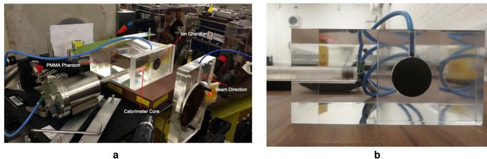
Figure 5. (a) The test-stand at the CLEAR facility, with the calorimeter, ion chamber and monitor chamber placed along the beam line with the beam travelling from right to left. The calorimeter core can be seen at the end of the PMMA sleeve (b). This shows the front surface of the custom PMMA phantom with Roos chamber insert placed to the right of the calorimeter sleeve. The PMMA build-up blocks, used to ensure the reference depth of the detectors was at 8 cm, are not included in the photographs.
