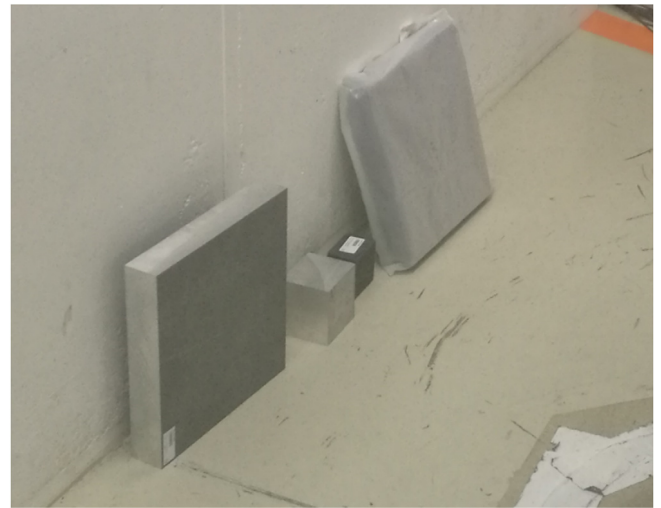
Fig. 4. Samples of aluminum and iron irradiated in CHARM.
