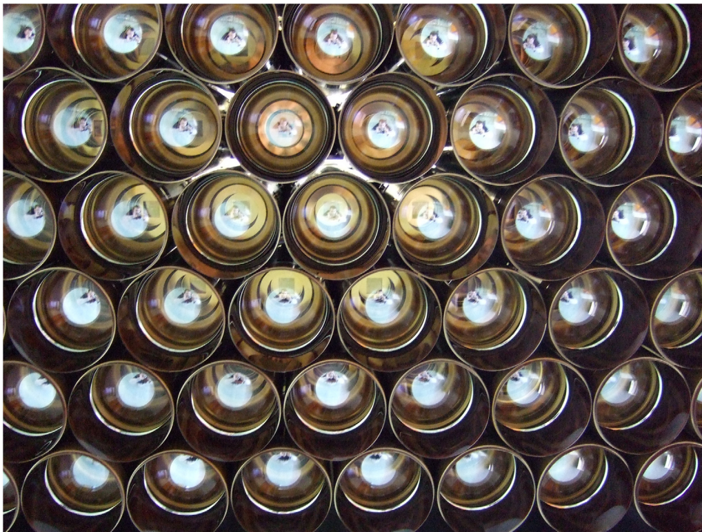
Fig. 24. Pixel-HPDs installed in the upper box of the LHCb-RICH 1 detector. Source: Picture source CERN.
