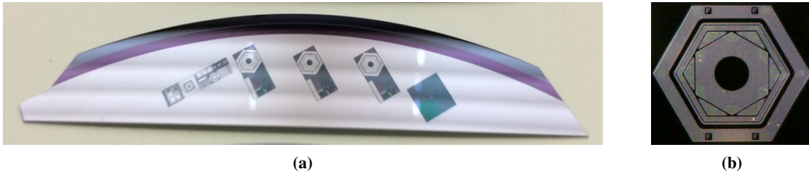
Figure 1. (a) Half moon sample with three test diodes and other test structures diced from an 8-inch Si wafer. (b) Close-up of the hexagonal test diode on the half moon sample. Corner to corner, the outer ring measures 4.5 mm.
