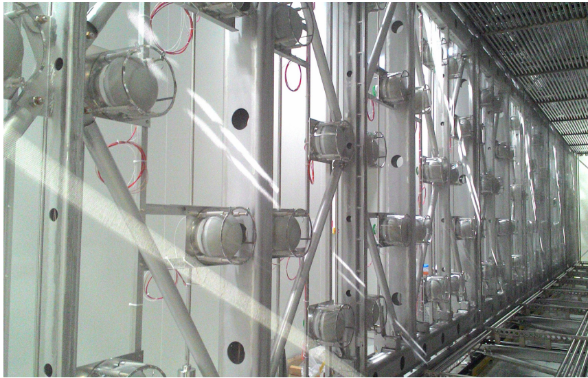
Figure 4. Scheme of the adopted geometry with 90 PMTs behind each wire plane and picture of the actual configuration.
