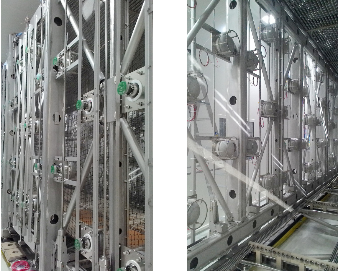
Figure 11. Picture of the PMT supporting system.
