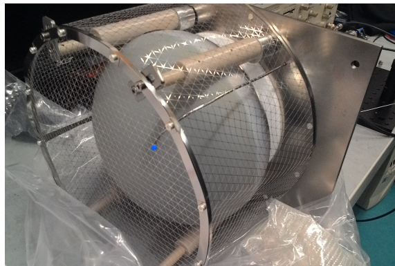
Figure 17. Picture showing the stainless steel pipe which drives the end section of the calibration optical fiber toward the PMT window. A blue-light laser spot on the PMT surface can be noticed.
