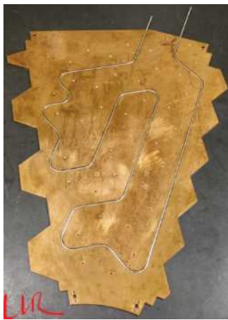
Pipe insertion on a cooling prototype
