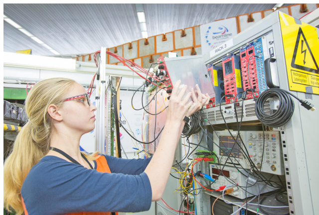
Fig. 11. Winning student of 2019 installing an electronics module in the trigger system (Image copyright: DESY/Marta Meyer).
