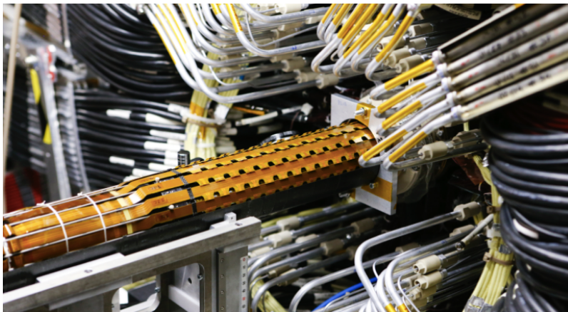
Figure 4. Image of the IBL being inserted (from left to right) into the pre-existing ATLAS Run 1 Pixel detector. A typical barrel structure divided in staves along the \phi coordinate is clearly visible in the picture.
