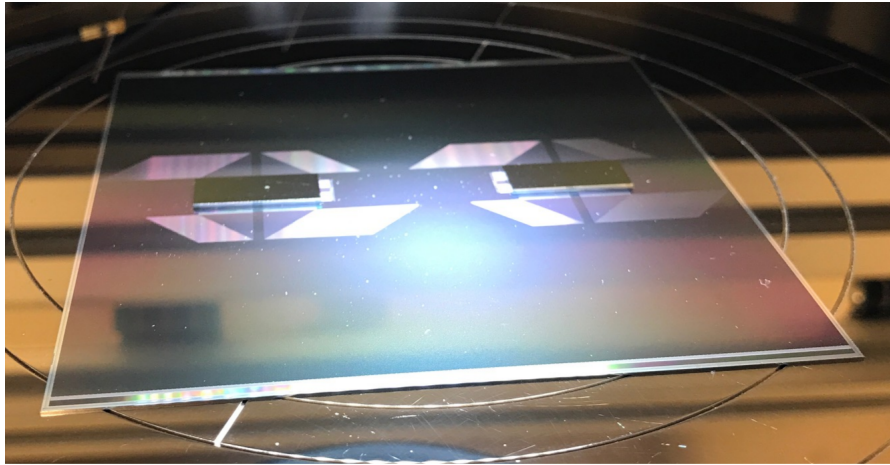
Figure 4: The SiD silicon strip sensor with two bump bonded KPix chips on the clean room probe station.
