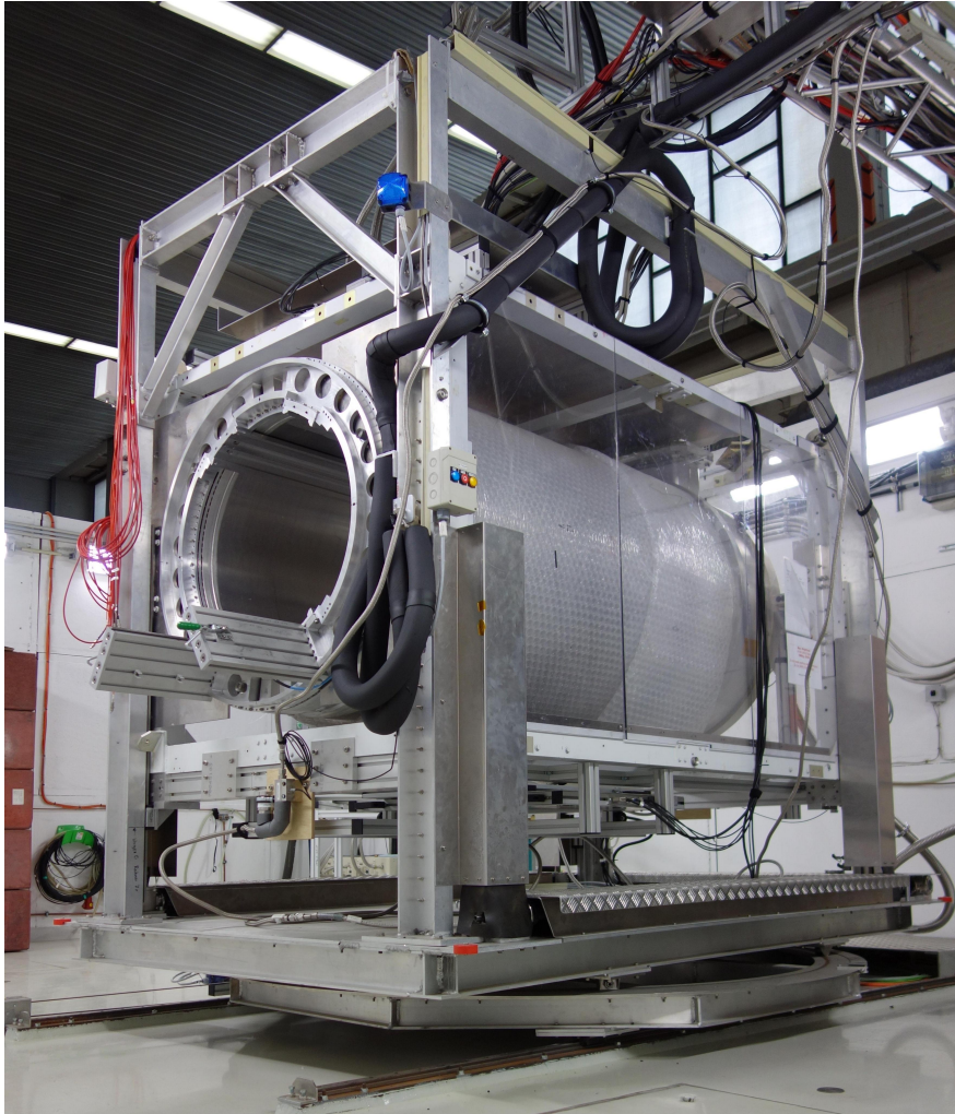
Figure 2: The PCMAG 1T solenoid mounted on the movable stage at DESY II test team area T24/1.
