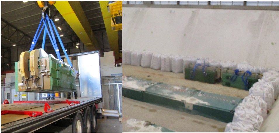
Fig. 11. Elimination of first electro-magnets as unitary pieces. Left figure: handling of magnet on the truck. Right figure: elimination in ANDRA's repository. Courtesy of ANDRA.
