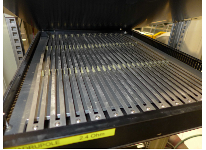
Figure 18: Resistor constructed from layers of thin sheets of stainless steel.
