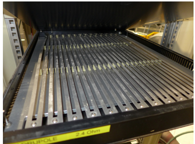
Fig. 16. Resistor constructed from layers of thin sheets of stainless steel, housed in a 1U rack-mount case. The resistor sheet is 12.25 inches wide and 20 inches deep.
