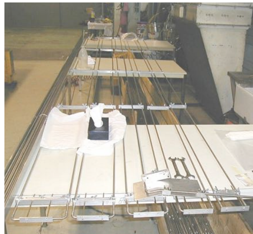
Figure 7. A few steps of the procedure to glue straight and U-shaped tubes.
